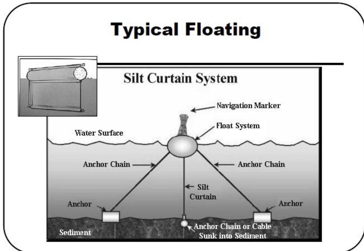
**Figure D-1. Typical Hanging Silt Curtain System**
