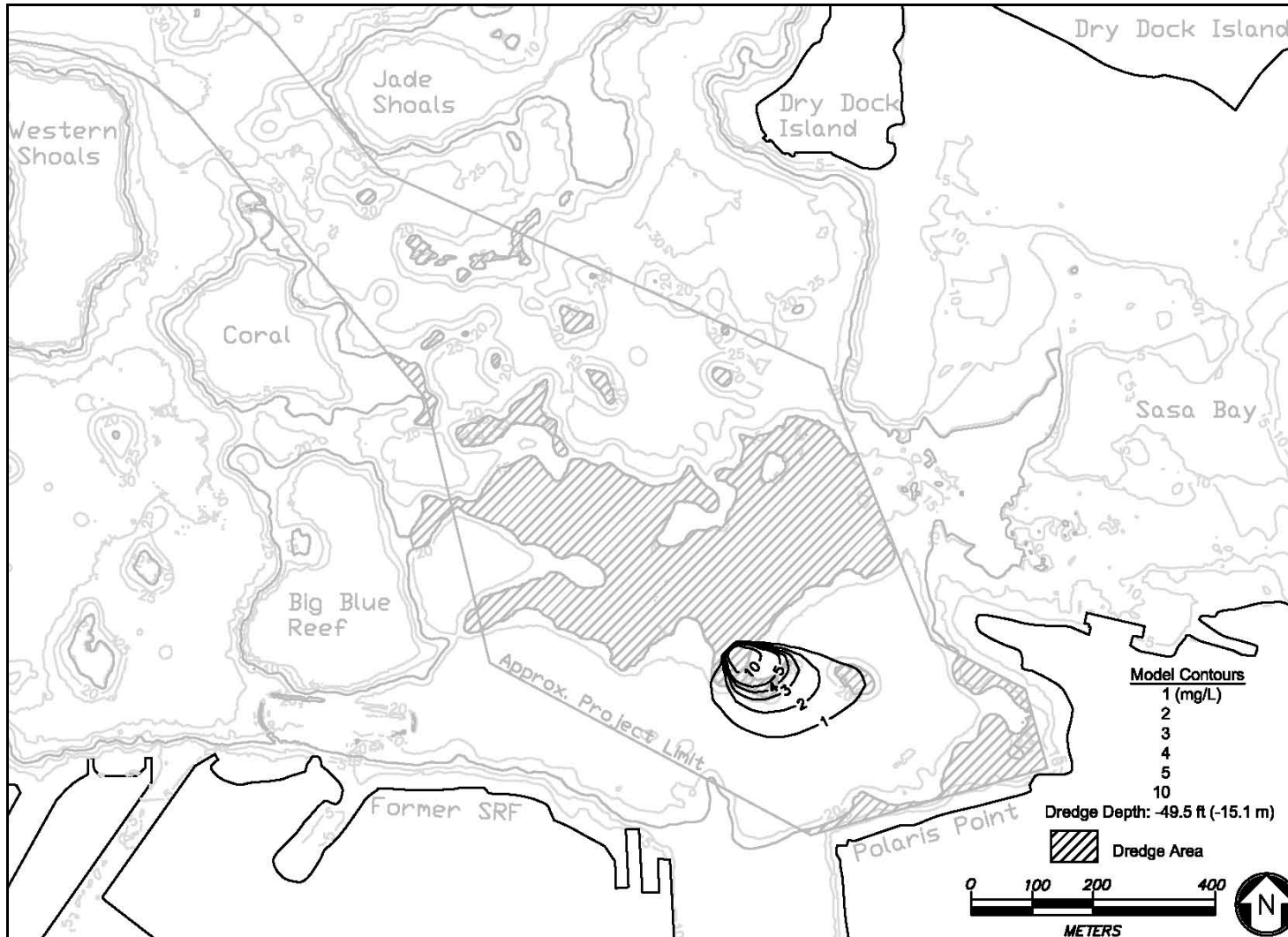
Figure 6-15B. Bottom Layer Suspended Sediment Concentration (6.15 December 15 to 18 winds, 10-hour dredging at D5)
