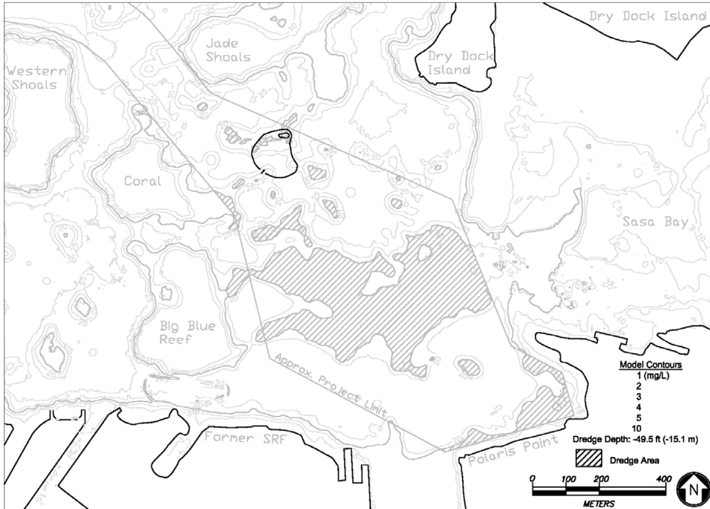
Figure 6-16A. Surface Layer Suspended Sediment Concentration (6.16 December 15 to 18 winds, 10-hour dredging at D6)
