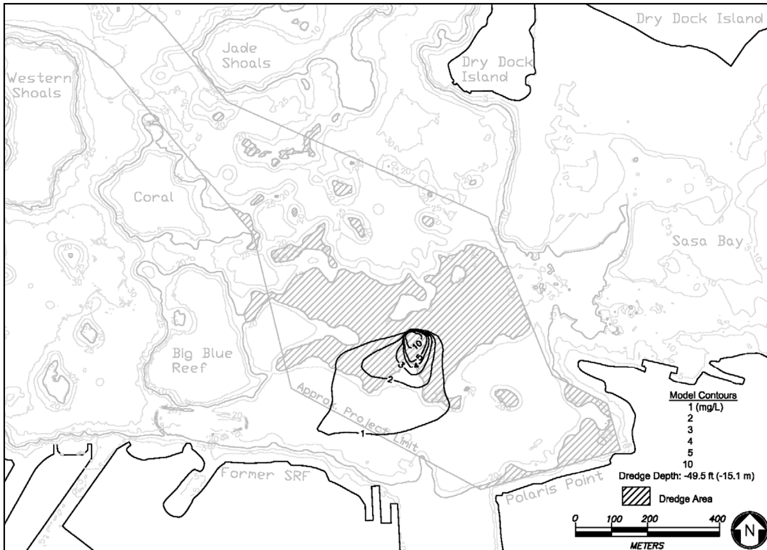
Figure 6-10D. Bottom Layer Suspended Sediment Concentration (6.10 Strong trade winds, 24-hour dredging at D1, Highest 10% release)
