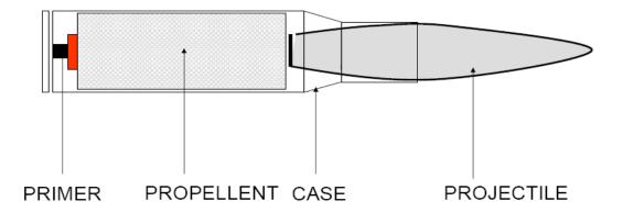
Figure D-5. Small Arms Cartridge Construction
