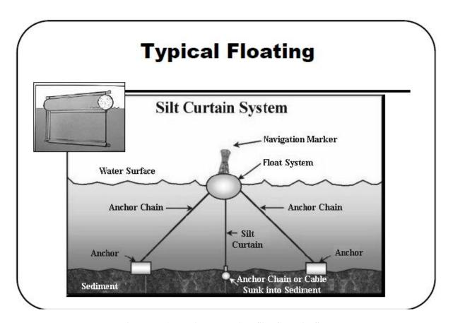
Figure D-1. Typical Hanging Silt Curtain System
