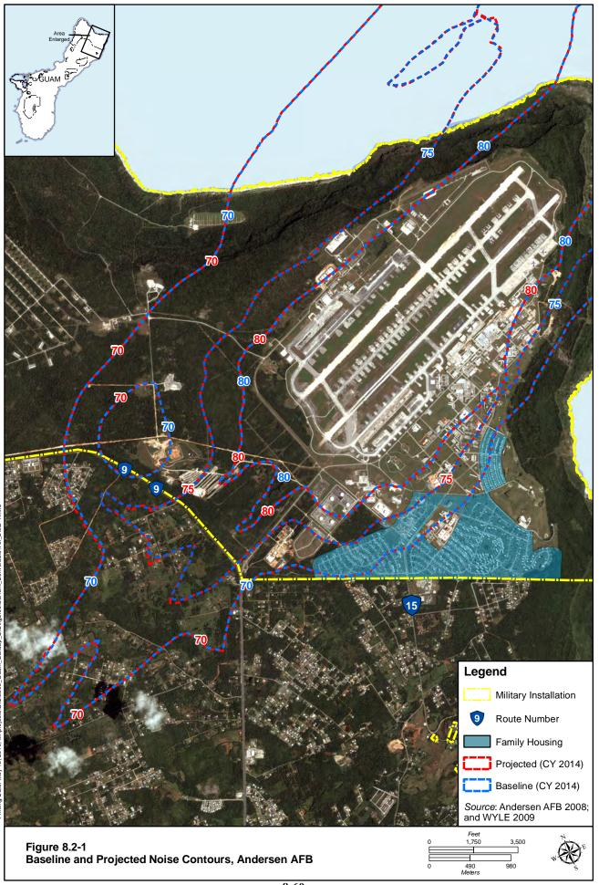
The noise contour for the Marine Corps aviation training at NWF and the operations at the main airfield of Andersen AFB is shown on Figure 6.2-1. The 60 decibel level contour extends slightly off base into the private coastal land located west of Andersen AFB, however 60 dB is relatively low and all land uses are compatible with this noise level. The impacts are considered less than significant.
